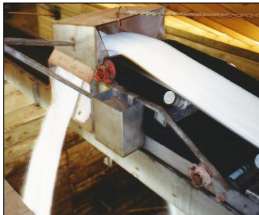
Overhead Conveyor with Gravity Tripper
